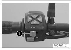
Turn signal switch **1** is fitted on the left side of the handlebar.
