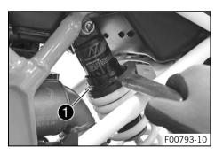
Adjust the spring pretension by turning adjusting ring 1. Guideline
