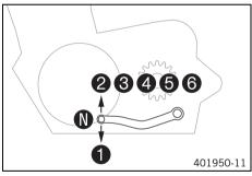
The gear positions can be seen in the photograph. The neutral or idle position is between the first and second gears.
