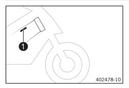
The type label USA 1 is located on the top frame on the right.
