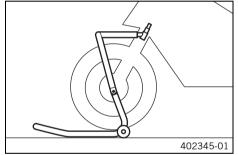
Move the handlebar to the straight-ahead position. Position the lifting gear.
