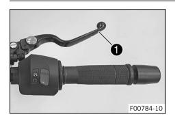
The hand brake lever **1** is fitted on the right side of the handlebar.
