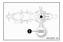
The USB diagnostics plug **1** is located under the combination instrument.
