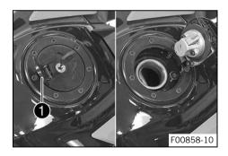
Lift cover 1 of the filler cap and insert the ignition key in the lock.
