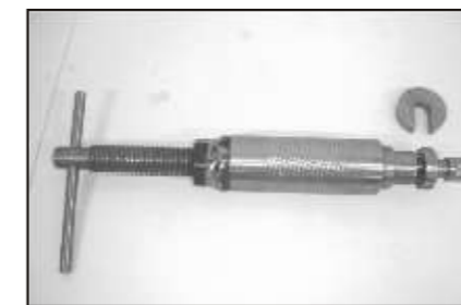
Needle Bearing Puller : Drawing No:74 9309 93 Application : To remove and refit needle roller bearing from swing arm.
