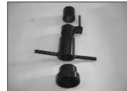
Fork Inner & Outer Tube Extractor: Drawing No:37 1740 04 Application : Used for removing front fork inner tube from outer tube.
