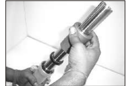
Fork Oil Seal Fitment Punch : Drawing No:37 1740 03 Application : To fit fork oil seal on outer pipe.
