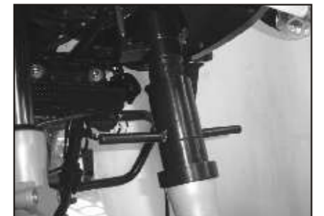
Fork Inner & Outer Tube Extractor: Drawing No:37 1740 04 Application : Used for removing front fork inner tube from outer tube.
