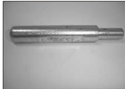
Drift Drawing No : 74 9309 89 Application : To remove piston pin.
