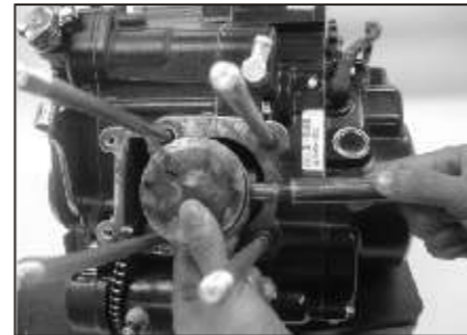
Drift Drawing No : 74 9309 89 Application : To remove piston pin.
