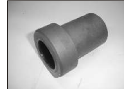
Fork Oil Seal Fitment Punch : Drawing No:37 1740 03 Application : To fit fork oil seal on outer pipe.
