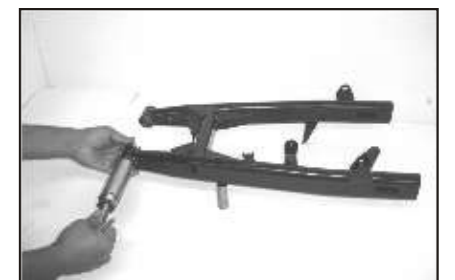
Needle Bearing Puller : Drawing No:74 9309 93 Application : To remove and refit needle roller bearing from swing arm.
