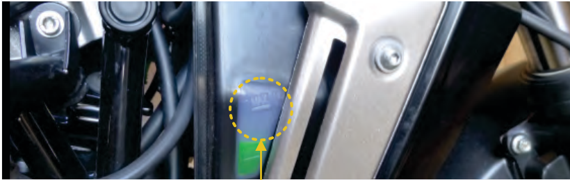
Coolant Expansion Tank
