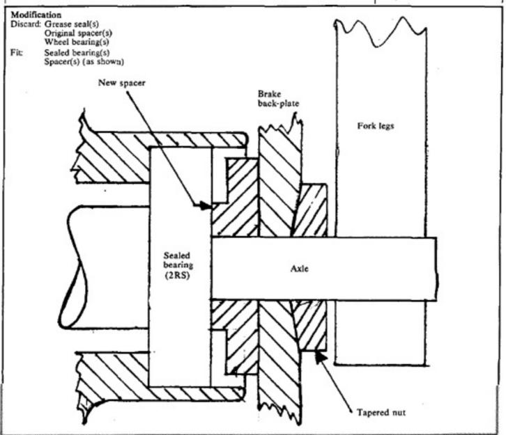
Royal Enfield brake backplate modification for 5in twin front brakes. Note: Spaces material stack. This is a general arrangement drawing orde.
