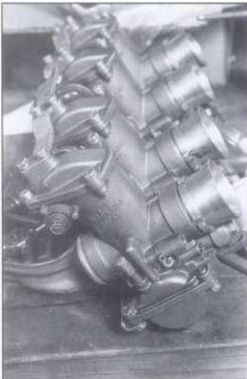
A rack of smoothbores for a 1025 Superbike engine. All carbs for multi-cylinder engines are rack-mounted because it simplifies slide synch, controls carb vibration, and it reduces throttle-spring tension. John Owens Studio
