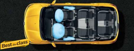
2 Front Airbags (Driver and Passenger) + 2 Side Airbags (Front Seats)
