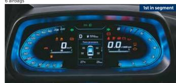
Tyre pressure monitoring system (highline) with display on MID
