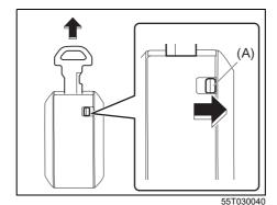
To remove the key from the remote controller, slide the lock knob (A) in arrow direc-
