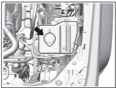
Check that there is washer fluid in the tank in the engine room. Refill it if necessary. Use a good quality windshield washer fluid, diluted with water as necessary.
