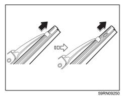
3) Unlock the lock end of the wiper blade and slide the blade out as shown.
