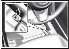
A fuel filler cap is located on the right rear side of the vehicle. The fuel filler door can be unlocked by pulling up the opener lever located on the outboard lower side of the driver's seat and locked by simply closing the door.
