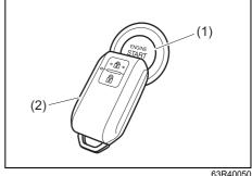
1) Manual transmission Without depressing the clutch pedal, push the engine switch (1).
