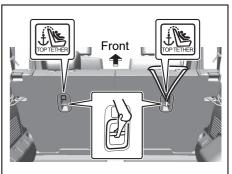
Some child restraint systems require the use of a top tether strap. Top tether anchorages are provided in your vehicle at the locations shown in the illustrations.
