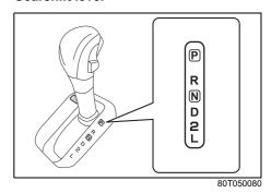
The gearshift lever is designed so that it cannot be shifted out of "P" position unless the ignition switch is in "ON" position and the brake pedal is depressed.
