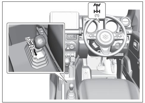
Shift the transfer lever without the lever pressed.
