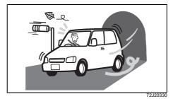
At a tunnel exit, on a bridge, or when a large truck passes you, your vehicle might be blown slightly sideways by side wind. Do not panic. Firmly grasp the steering wheel, gradually reduce speed, and regain your intended course.
