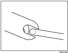
4) Push the child restraint toward the anchorages so that the connecting bar tips are partially hooked to the anchorages. Use your hands to confirm the position.
