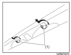
1) Remove the cover (1) by turning it counterclockwise.
