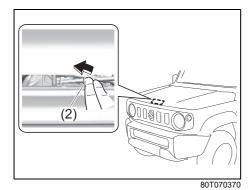
2) Push the under-hood release lever (2) sideways with your finger, as shown in the illustration. While pushing the lever. lift up the hood.
