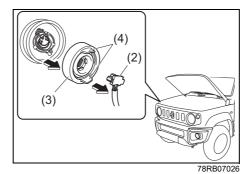
Open the engine hood while the engine is stopped. Disconnect the coupler (2). Remove the sealing rubber (3) by pulling the grip (4).
