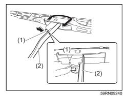
Squeeze lock (1) towards wiper arm (2) and remove the wiper frame from the arm as shown.
