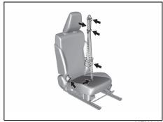
Periodically check if the seat belts work properly and are not damaged. Check the webbing, buckles, latch plates, retractors, anchorages and guide loops. Replace any seat belts which do not work properly or are damaged.
