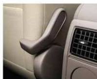
Ergolever for front passenger seat adjustment from the rear
