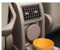
Adjustable dual rear air conditioning vents
