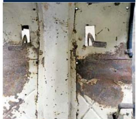
The pedal on the left is the rear brake, while the two on the right are for going through the gears, with the toe changing to first while the heel does the others.
