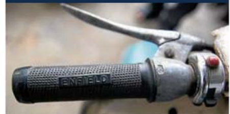
Adjacent to the left grip is the red electric starter button and the black headlamp switch.
