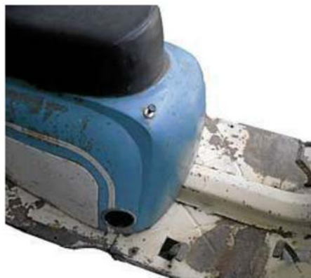
The choke button on Muthu's 1962 scoot is near the seat, but later models had it on the dash.
