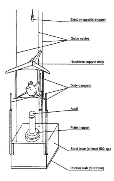
Fig. 1 TEST MACHINE HEADFORM DROP ASSEMBLY
