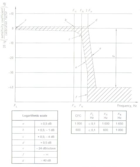
Figure 1 — Frequency response limits — CFC 1000 and CFC 600
