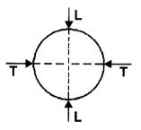
**7.3.2.2** The load applied to the plates shall then be reduced to 30 N at a minimum plate speed of 20 mm/min and kept at that value for five minutes, the distance between the plates shall then be measured.
