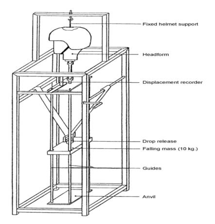
Fig. 1 DYNAMIC TEST OF RETENTION SYSTEM
