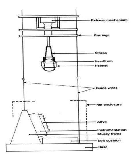
Example of a Suitable Test Apparatus for Projections and Surface Friction (Method A)
