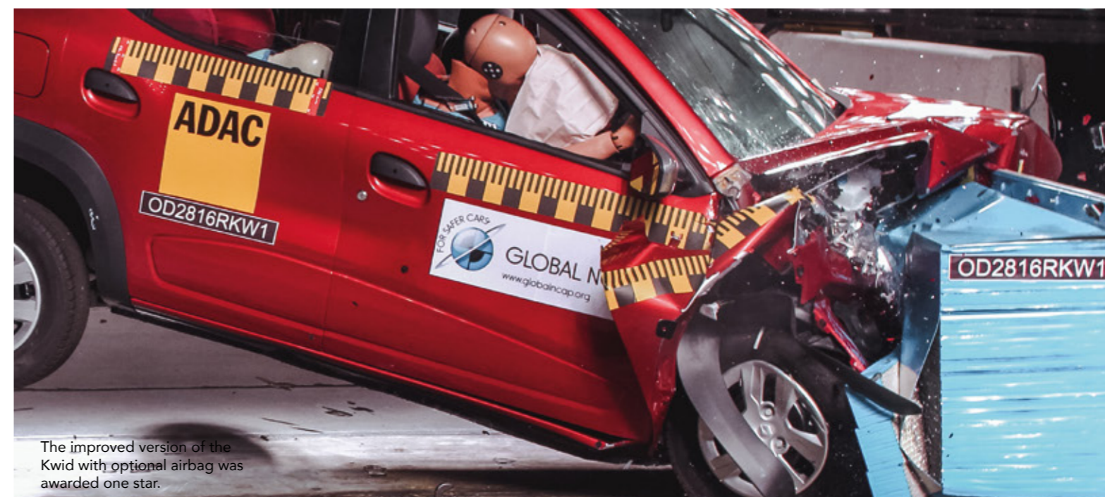
The first Renault Kwid tested by Global NCAP scored zero as the bodyshell collapsed.
