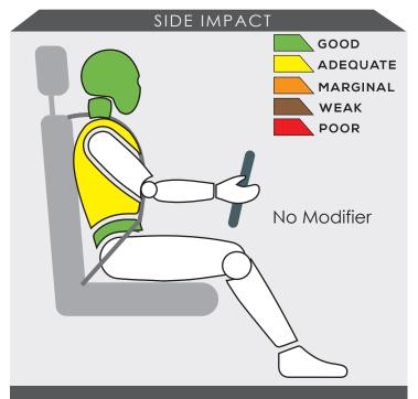
Data obtained showed the driver's chest had adequate protection during the side impact test.
