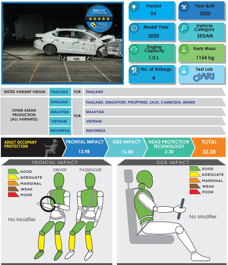
The car's frontal occupant compartment remained stable in the frontal offset test. The data obtained from the test revelaed that the vehicle gave a good protection to both of the adult occupants, with an exception to the dummies' lower legs. The performance of HPT was confirmed with additional deployment test and its score was determined based on Fitment Rating System (FRS).
