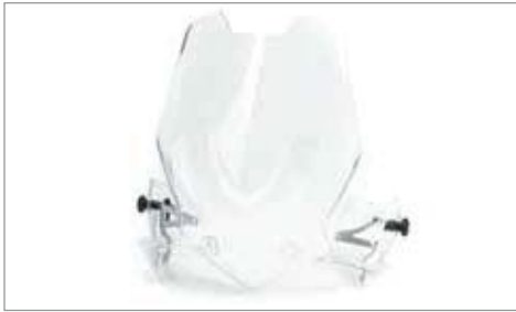
ADJUSTABLE HIGH SCREEN KIT ✂ 0.5 Injection moulded polycarbonate screen with adjustable mount. 53mm higher and 55mm wider than OE. Tilt angle adjustment of 12.4 degrees (47mm). No tools required to adjust tilt angle. A9708248
