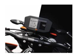
» A state-of-the-art full color TFT display offers variable configuration and automatically adapts to variations in environmental light. Changing colors in the rev counter are used to indicate when to shift. The rider can select which information is displayed on the screen. For example: trip meter, fuel range, etc. The overall objective was to achieve easy readability; the main information is arranged in a position where the rider can immediately see it.
