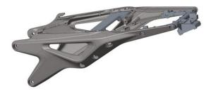
» The subframe is cast aluminum. and houses the airbox. No plastic covers, no additional brackets everything is cast in one single piece to reduce complexity and weight. The triangular shapes in the subframe were inspired by KTM's trellis subframes, as this allows for a strong and simple construction.
