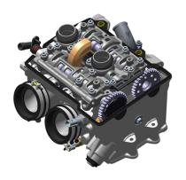
» Offering decreased rotating mass for smooth performance, The cylinder head contains twin chain driven camshafts that open the valves by DLC coated finger followers riding on the cam to reduce the size of the cam lobes, decreasing rotating mass.
