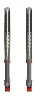
» The 790 Duke is fitted with 43mm open cartridge upside down front forks from WP Suspension. The fork uses split function technology, with compression and rebound damping taking place in separate fork legs, allowing for better tuning of the fork behavior. Fork springs are progressive, ensuring a smooth operation throughout the fork stroke, soft for the initial stroke and harder further down the stroke to prevent bottoming out.
