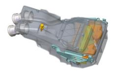
» The airbox sits entirely inside the sub-frame, with separate air intakes on both left and right sides, allowing fresh air to enter into the throttle body. This location also provides easy air filter maintenance.
