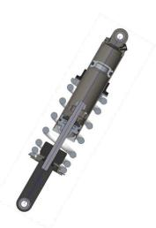
» To complement the highquality WP forks fitted to the front of the 790, a gas assisted WP Suspension rear shock with progressive spring and preload adjustment was added to the rear. The shock is mounted directly to the swingarm with no linkage, reducing additional parts and weight.
