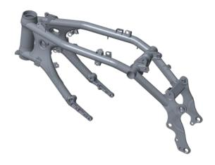
» The frame has been developed with a focus on weight reduction. By using Chromium Molybdenum tubular steel and the engine as load-bearing element in the frame, the amount of material needed for a strong and stiff frame is reduced. The stiffness of the frame has been tuned to make sure that the rider always feels what the bike is doing.
