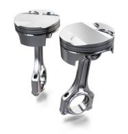
» Designed to be light for fast revving and reduced vibration, the lightweight forged pistons utilize a DLC (Diamond Like Carbon) coated piston pin that allows for a reduced piston weight and thus reduced reciprocating mass. They are connected to the crankshaft by a forged and cracked conrod in plain bearings. The cracked conrod doesn't require locating dowels, further reducing assembly weight.
