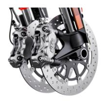
» Stopping power is guaranteed by twin 300mm floating disks, 4 piston radially mounted calipers controlled by a radial master cylinder. The brakes have been developed specifically for the 790 DUKE to provide excellent feedback while ensuring sporty deceleration.
