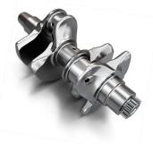
» Built to be light while robust, the one-piece, forged crankshaft with plain bearings is designed to reduce rotating mass and has a 75° conrod journal position to produce engine character similar to the large V-twin LC8.
