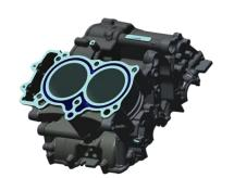
» Nikasil coated aluminum cylinders are an integral part of the sleeveless engine casing. The open deck cylinder construction allows for optimal cooling, due to the coolants ability to make full contact with the surface area of the upper portion of the cylinder, improved production tolerances and reduces the potential for cylinder warpage during production.
