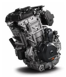
» The most compact engine in its segment, the LC8c (Liquid Cooled 8 Valve compact) is KTM's first parallel twin. The engine was built for torque, to give the rider usable power from low RPM while still giving that top-end rush. It has 799 cc with a 75 degrees crankpin and a DOHC.
