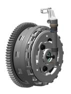
» The PASC (Power Assist Slipper Clutch) clutch is similar to the one in the LC8, but more compact and lighter. The clutch is pressure lubricated for improved cooling and reduced friction. Not only does the slipper clutch open when the engine back-torque becomes too high, it also assists when you open up the throttle, reducing the force required to pull the clutch in and allowing the clutch to be operated with as little as one finger.
