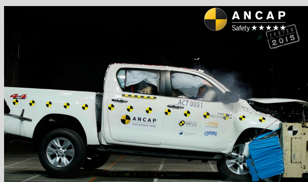
Frontal Offset test at 64km/h (Toyota Hilux tested)
