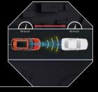
Adaptive Cruise Control is an advanced version of cruise control. It senses and monitors the road ahead and automatically accelerates/decelerates for maintaining a proper distance from the vehicle in front.
