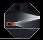
Intelligent Headlamp Control activates and deactivates the high-beam, depending on the oncoming traffic and environment situation. Thus preventing other road users from blinding due to high-beam.
