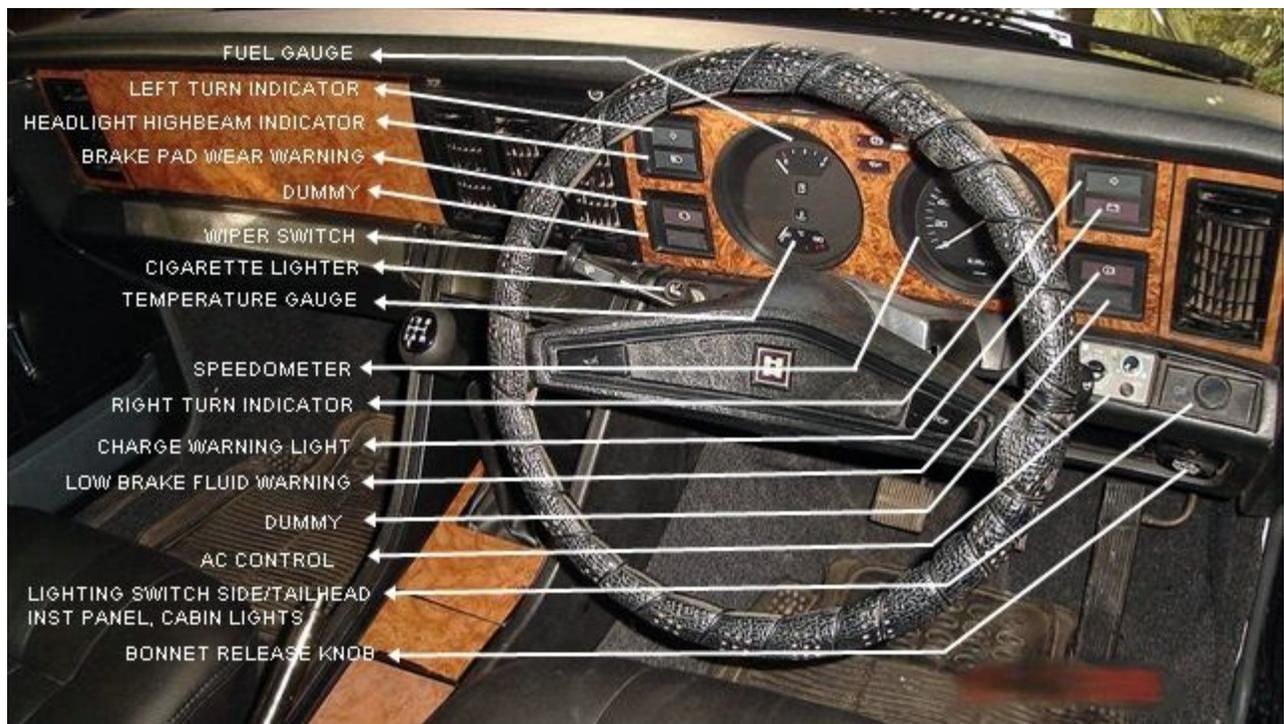
This is a picture of the Contessa Classic1.8 Dashboard, Instrument Cluster and Controls. The description of each control is marked with an arrow.
