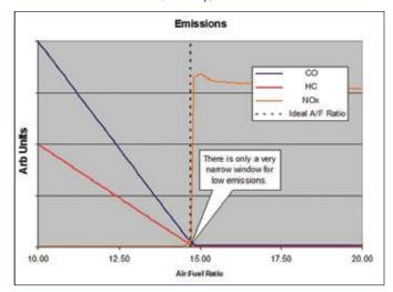
Figure 2: Reducing nasty emissions is the other job of the ECU, but it's tough. As the air/fuel ratio increases, carbon monoxide and hydrocarbons are reduced, but go just over the ideal air/fuel ratio in search of better fuel economy, and NOx suddenly skyrockets.
