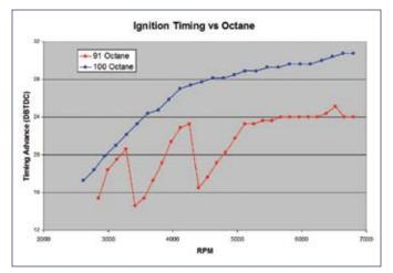
Figure 3: Knocking, caused by using poor quality gasoline, or pushing the engine too hard, is controlled the ECU by reducing the timing of the spark, which allows the gas more time to burn. Unfortunately, as shown here comparing acceleration with high octane and low octane gasoline, the changes in timing are abrupt and substantial, causing poor performance.
