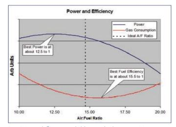
Figure 1: Power and efficiency can not both be improved at the same time. Maximum power is achieved with more fuel and less air, while fuel efficiency gets better up to a point as the air to fuel ratio increases. The ECU works to keep the best proportions under different modes of operation.
