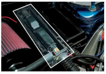
The ECU exposed: The ECU is next to the air intake. With the cover removed, the wires going into the engine compartment can be seen at the front, and the connector into the passenger compartment at the rear. The computer itself is just below the connectors.
