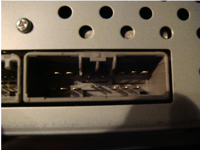
System connector #1 (power, car speaker signals, and some other bits)
