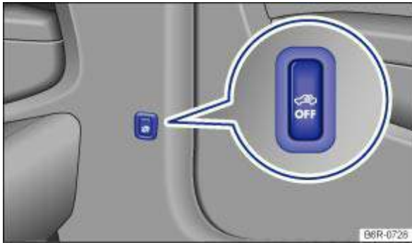
Fig. 29 Next to the driver seat: button for switching off the interior monitoring system and anti-tow alarm
