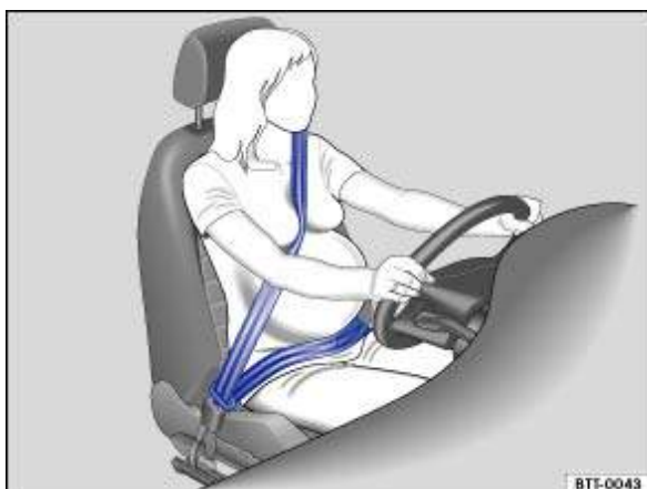
Fig. 57 Correct seat belt routing during pregnancy
