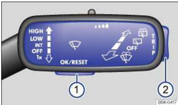
Fig. 15 Vehicles without a multifunction steering wheel: button ① on the windscreen wiper lever for confirming menu points, and rocker switch ② for changing menus and information displays
