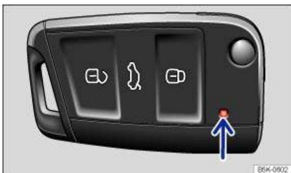
Fig. 23 Indicator lamp in the vehicle key
