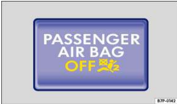
Fig. 59 In the upper section of the centre console: indicator lamp for disabled front passenger front airbag
