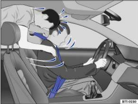
Fig. 52 The unbelted rear passenger is thrown forwards, hitting the belted driver
