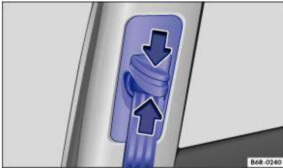
Fig. 58 Next to the front seats: belt height adjuster
