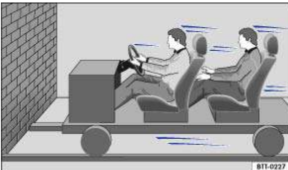
Fig. 49 Unbelted occupants in a vehicle heading for a brick wall
