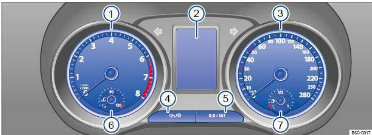
Fig. 11 Instrument cluster in the dash panel (variant 2)
