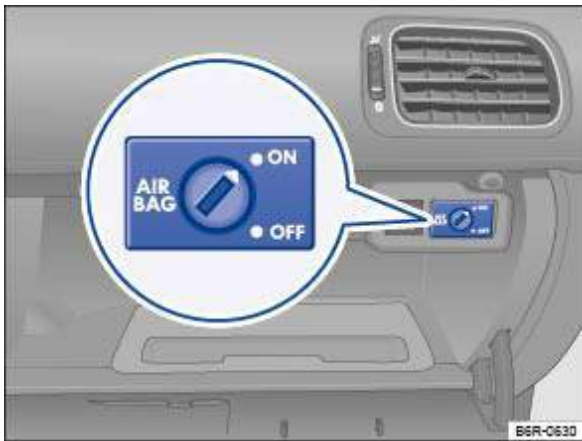
Fig. 62 In the stowage compartment on the front passenger side: key switch for disabling and enabling the front airbag on the front passenger side
