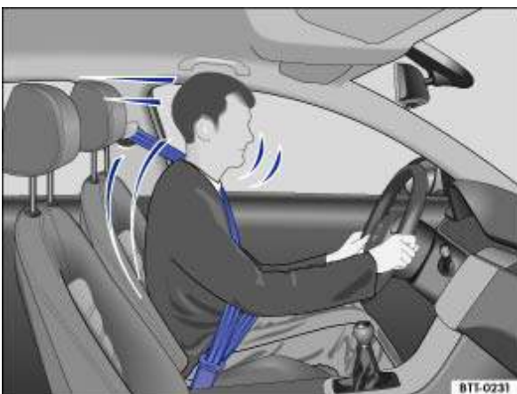
Fig. 53 Driver restrained by a properly positioned seat belt during a sudden braking manoeuvre
