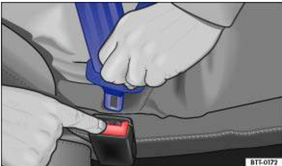
Fig. 55 Removing the latch plate from the buckle
