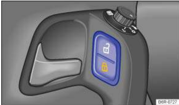
Fig. 28 In the driver door: central locking button
