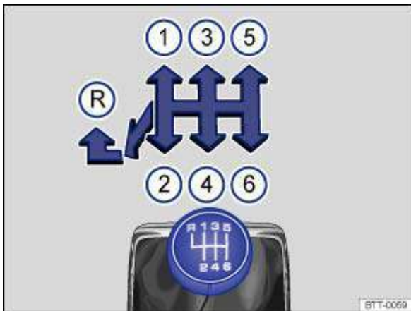
Fig. 115 Gear shift pattern of a 5 or 6-speed manual gearbox (variant 1)
