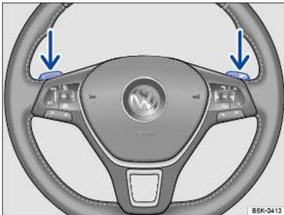
Fig. 120 Steering wheel with two paddles for Tiptronic
