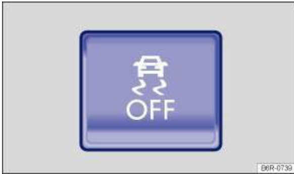
Fig. 123 In the upper part of the centre console: button for switching TCS, TCS with ESC or ESC Sport on and off manually
