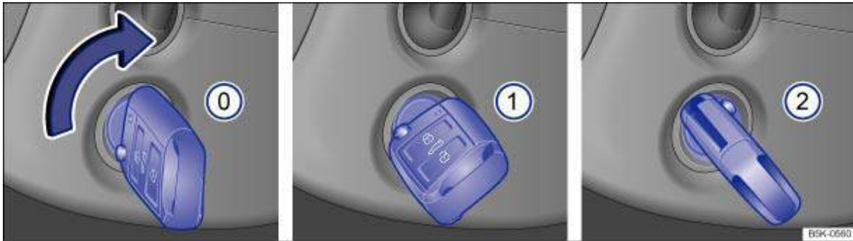
Fig. 112 Positions of the vehicle key in the ignition lock
