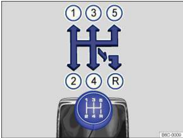
Fig. 116 Gear shift pattern of a 5-speed manual gearbox (variant 2)
