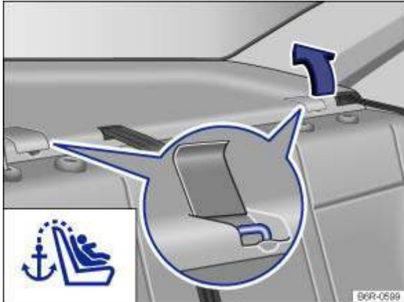
Fig. 70 Retaining ring for top tether in the stowage area behind the rear seats
