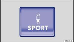
Fig. 152 In the upper section of the centre console: button for setting the "Sport Select" chassis
