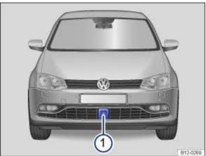
Fig. 143 In the front bumper: radar sensor
