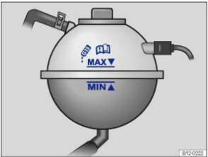
Fig. 166 In the engine compartment: mark on the coolant expansion tank
