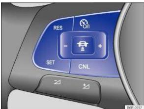
Fig. 144 Left-hand side of the multifunction steering wheel: buttons for operating the Adaptive Cruise Control (ACC)
