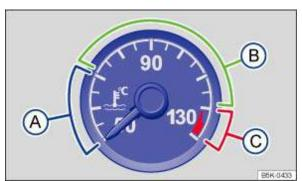
Fig. 165 Coolant temperature display in instrument cluster: (A) cold; (B) normal; (C) warning
