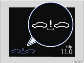
Fig. 147 On the instrument cluster display: distance warning display
