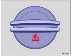
Fig. 167 In the engine compartment: coolant expansion tank cap
