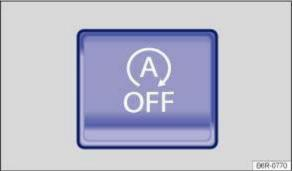
Fig. 127 In the upper part of the centre console: button for the start/stop system
