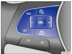
Fig. 140 Left-hand side of the multifunction steering wheel: buttons for operating the CCS
