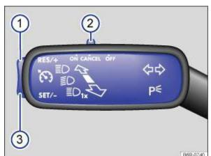
Fig. 139 On the left of the steering column: switch and buttons for operating the CCS
