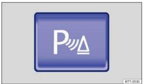
Fig. 129 In the upper section of the centre console: button for switching the ParkPilot on and off
