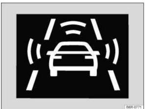
Fig. 148 The display in the instrument cluster: advance warning display
