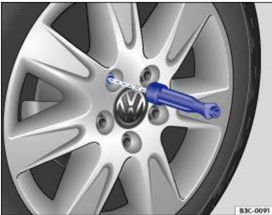
Fig. 201 Changing the wheel: removing the wheel bolts with the screwdriver handle
