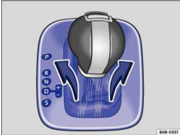
Fig. 187 Removing the cover of the gearshift gate (left-hand drive) The controls are mirrored in right-hand drive vehicles
