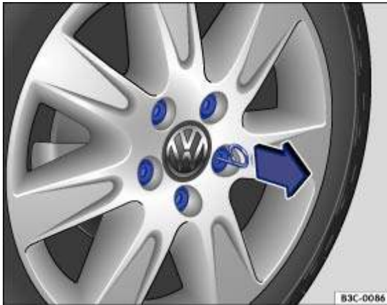
Fig. 194 Removing the wheel bolt caps
