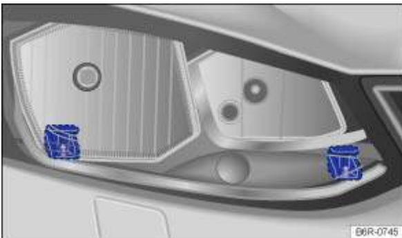
Fig. 210 Guides for installing the right headlight
