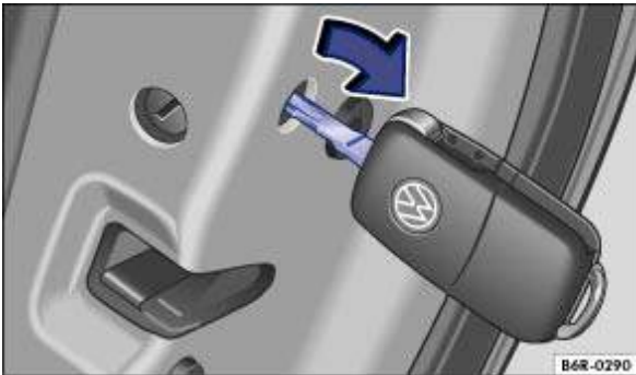
Fig. 185 Manually locking the vehicle with the vehicle key
