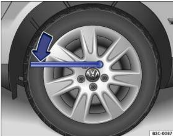
Fig. 195 Changing a wheel: loosening the wheel bolts
