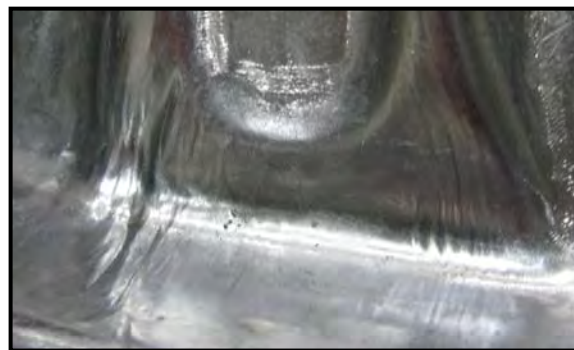
Figure 3.C-7: Draw die with significant wear due to excessive wrinkling on a DP780 part.
