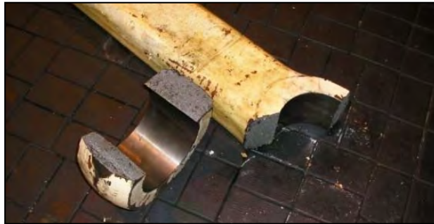
Figure 3.C-57: Broken connecting rod on a mechanical press. M-5
