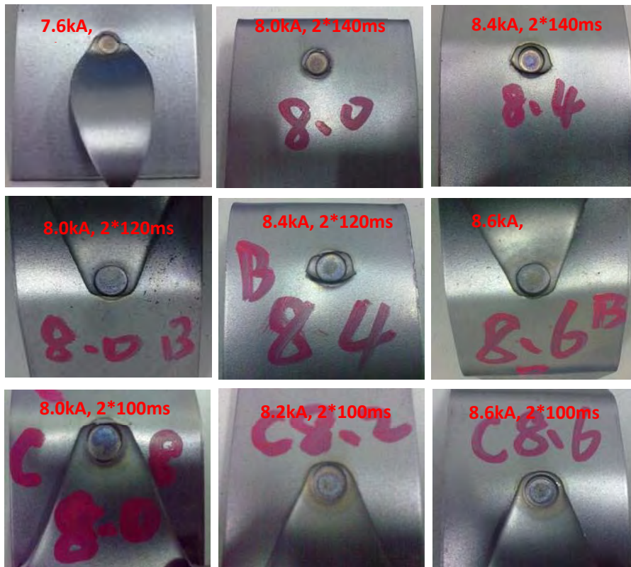
Figure 4.C-13: Fracture mode of weld spots in yellow zone. B-4
