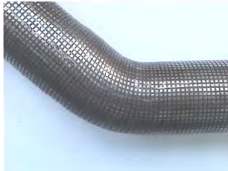
Figure 3.E-10: Bending test of welded DP 350/600 tube with YS \approx 610 N/mm 2 ; TS \approx 680 N/mm 2 ; Total Elongation \approx 27%. Booster bending, Centerline Bending Radius = 1.5 x D, Bending Angle = 45 Degrees. R-1
