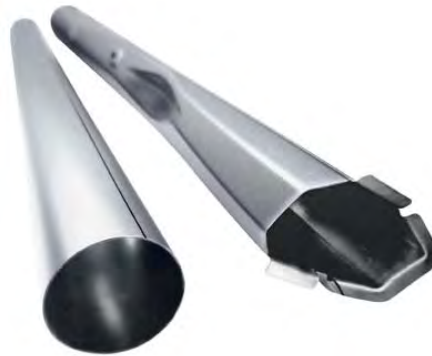
Figure 3.E-13: Front-rail prototype based on a conical tube having 40 mm end to end difference in diameter. F-2
