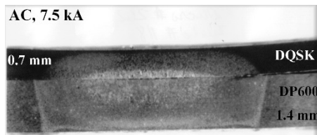
(a) Insufficient fusion at the interface with AC power source.
