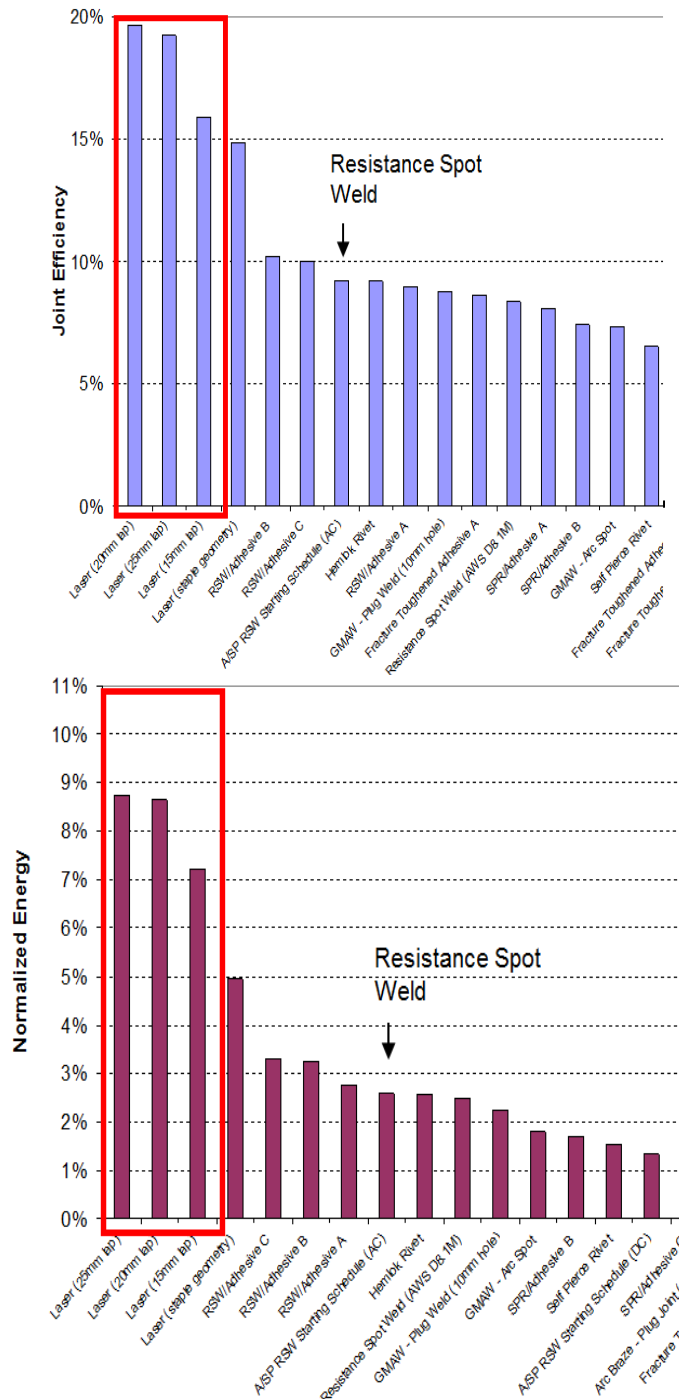
Figure 4.S-6: Joint efficiency and normalized energy of DP 600 lap shear for all processes. A-12
