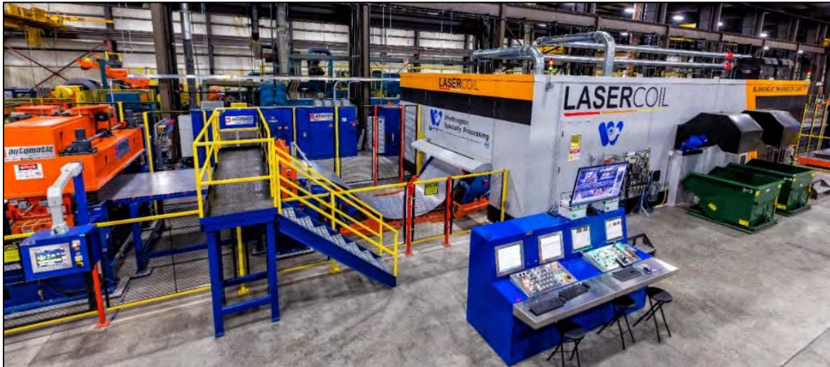
Figure 3.E-5: Laser blanking line specifically designed to process AHSS. As described in Section 3.C.7. – Straightening and Precision Leveling AHSS, there is even a cartridge designed straightener (far left) specifically designed to insure blanks are flat after processing.
