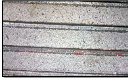
Figure 3.C-48: Slit edges on a lift of blanks that successfully produced DP980 rocker panels. Note the uniform transition from the burnish zone to the fracture zone with a smooth fracture zone as well. M-7
