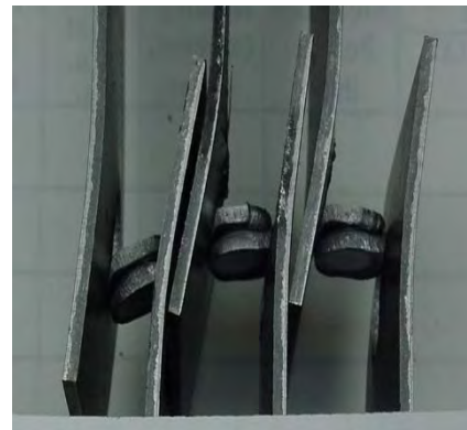
(b) Fracture by button pull out (high currents)
