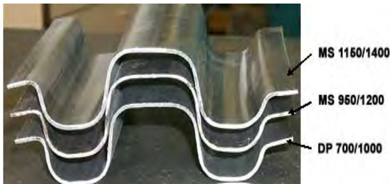
Figure 3.B-55: Profile made with the same tool setup for three different steels. S-5
