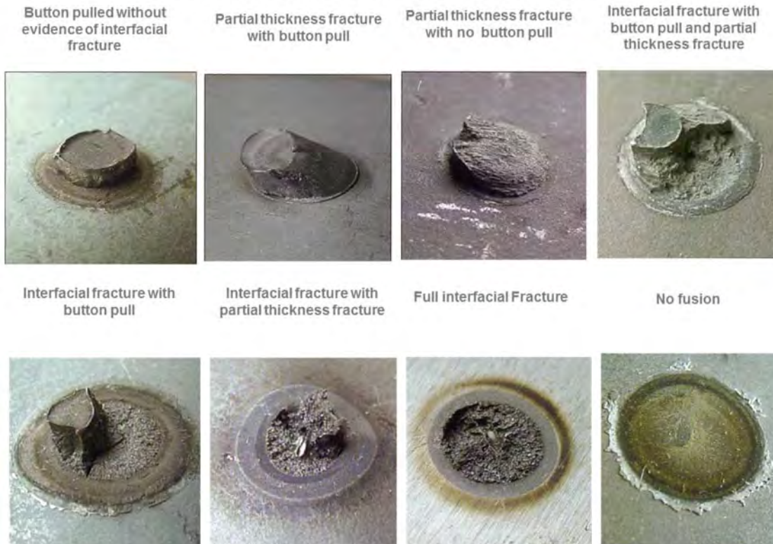
Figure 4.D-14: Peel and chisel test fracture modes in automotive industry.
