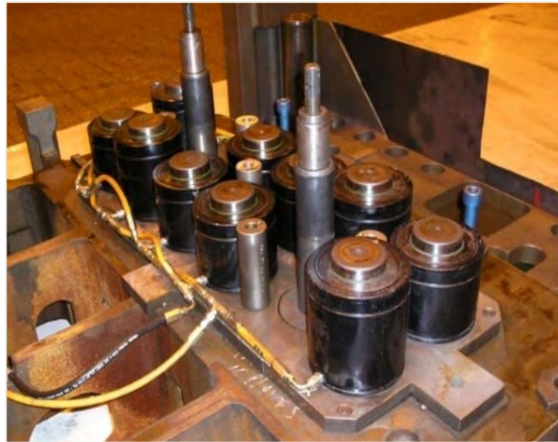
Figure 3.C-67: Staggered nitrogen cylinders designed to reduce the initial shock load when setting draw beads by engaging at different depths in the press stroke. M-5
