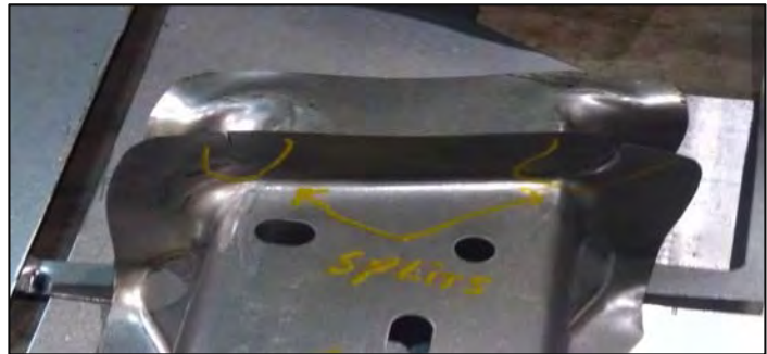
Figure 3.C-4: Edge fractures transferred from the draw die to flange die.
