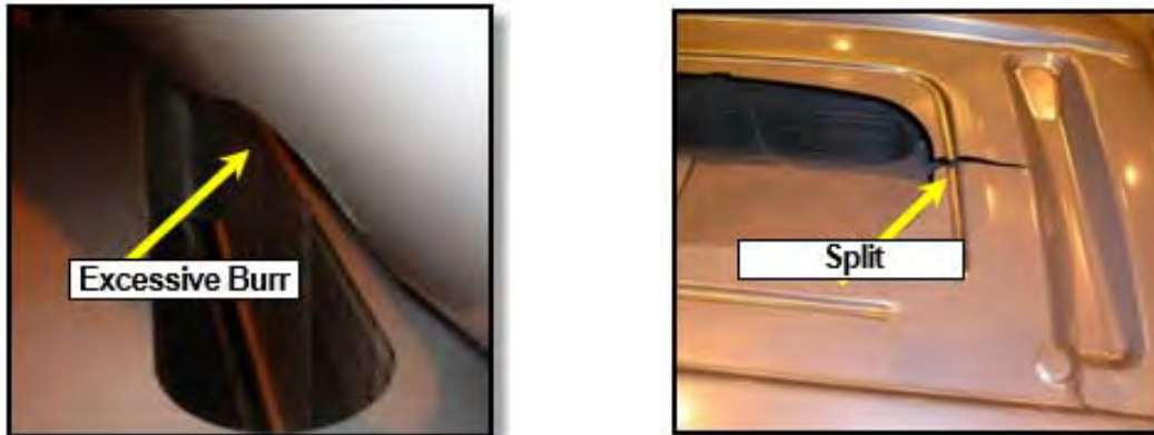
Figure 3.C-44: Excessive burr on blank (top) and a global formability split on the formed liftgate (bottom) due to excessive work hardening. Dull trim steels were the cause of this condition. M-8
