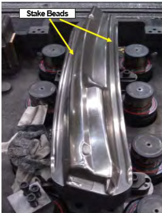
Figure 3.C-26A: Stake beads machined into the punch of this DP780 die.
