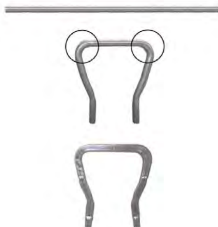
Figure 3.E-16: This duplicate of Figure 3-167 shows the two potential problem areas (circled) for a hydroformed Engine Cradle made from welded DP 280/600 tube . R-1
