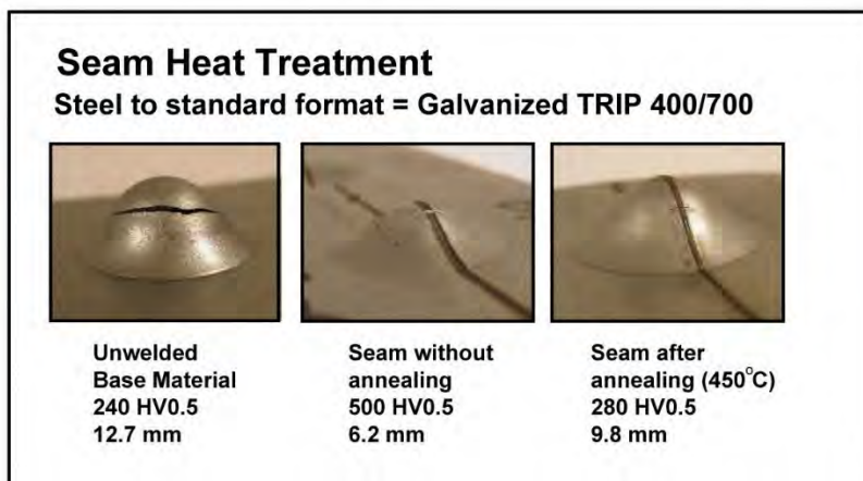
Figure 4.J-9: Improved stretchability of AHSS laser welds with an induction heating post-Heat treatment (Testing performed with Erichsen cup test T-3 )
