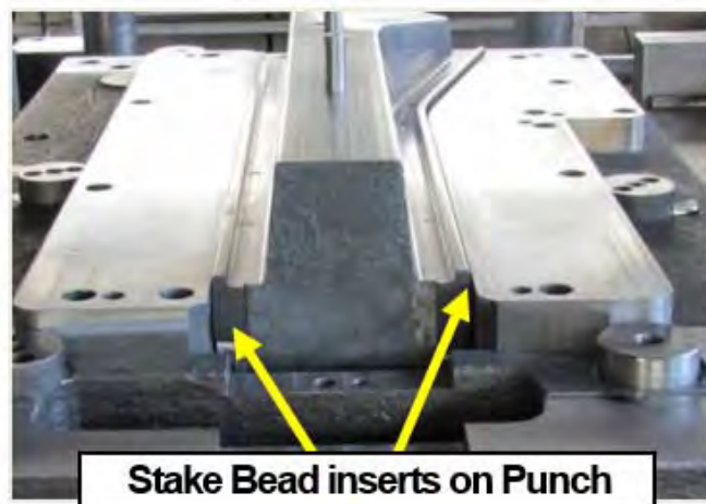
Figure 3C-27: This die has adjustable stake beads, but they are located on the punch as inserts and do not retract during every press stroke. Note also that there are no draw beads on the blankholder.
