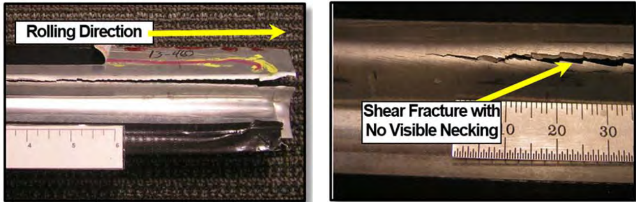
Figure 3.B-30: Shear fracture running in the rolling direction (left). Close-up of the same shear fracture (right) where the fracture is on the radius, not on the tangent to the radius. Note also there is no sign of thinning or necking at the fracture. M-5
