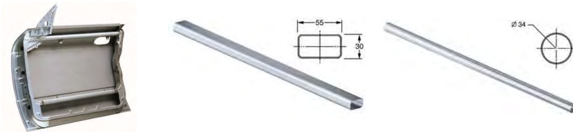
Figure 3.E-6: ULSAC study door (left) and DP500/800 lower (center) and outer belt reinforcement tubes (right)
