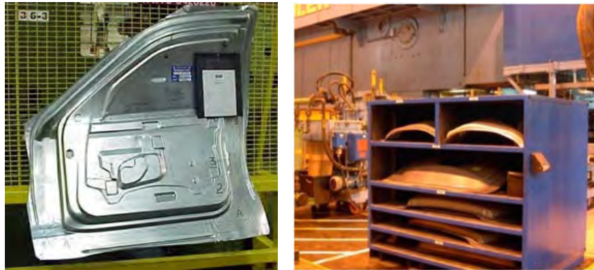
Figure 3.F-2: Door Outer Reference Panel and Storage Rack
