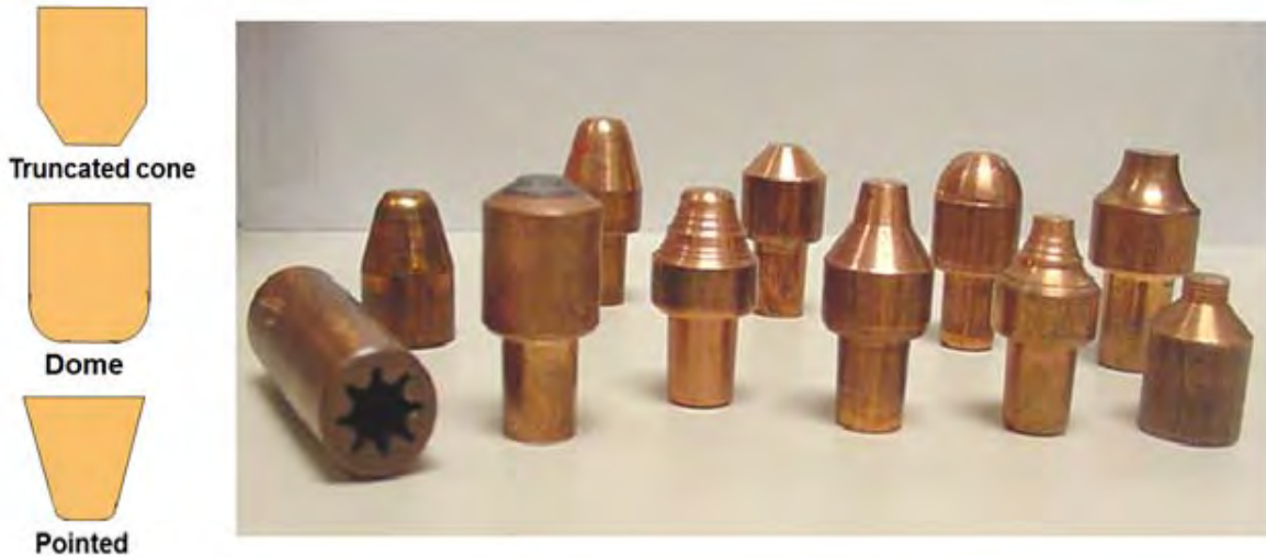
Figure 4.C-5: Typical RSW electrode geometries (left), example geometries used by automotive manufacturers (right).
