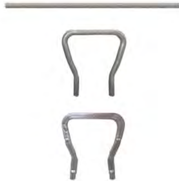
Figure 3.E-9: Hydroformed Engine Cradle made from welded DP 280/600 tube with YS \approx 540 N/mm 2 ; TS \approx 710 N/mm 2 ; Total Elongation \approx 34%. Draw bending, Centerline Bending Radius = 1.6 x D, Bending Angle > 90 Degrees. R-1
