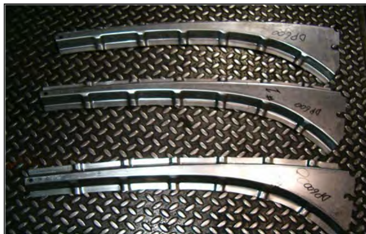
Figure 3.C-42: DP600 front rail upper reinforcements with vertical beads designed into the part geometry to help control springback.
