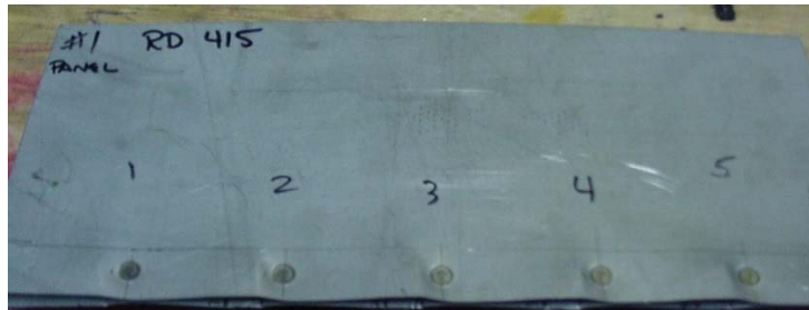
Figure 4.D-6: Semi-destructive chisel testing in 0.8-mm DP 300/500 EG. M-1
