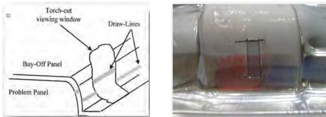
Figure 3.F-3: Draw-in template for draw panel; cutout allows for accurate, repeatable measurement.
