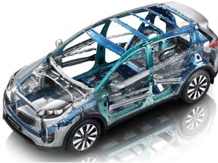
Figure 1.D-4: Kia Sportage body structure is 51% AHSS. K-8
