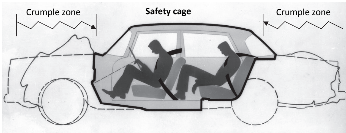
Figure 8.1: The major crash management zones of a vehicle [Adapted from 18]
