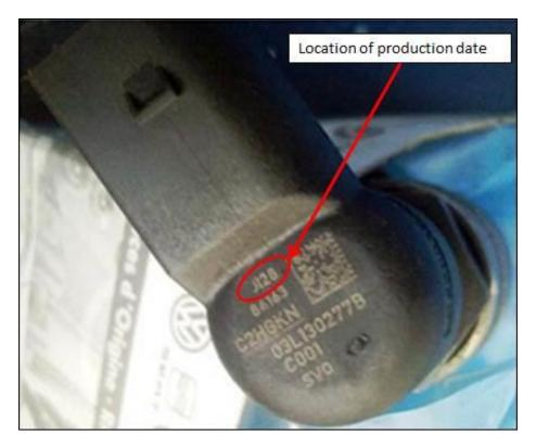
Defective injector must be replaced by improved injector as per following guidelines:
