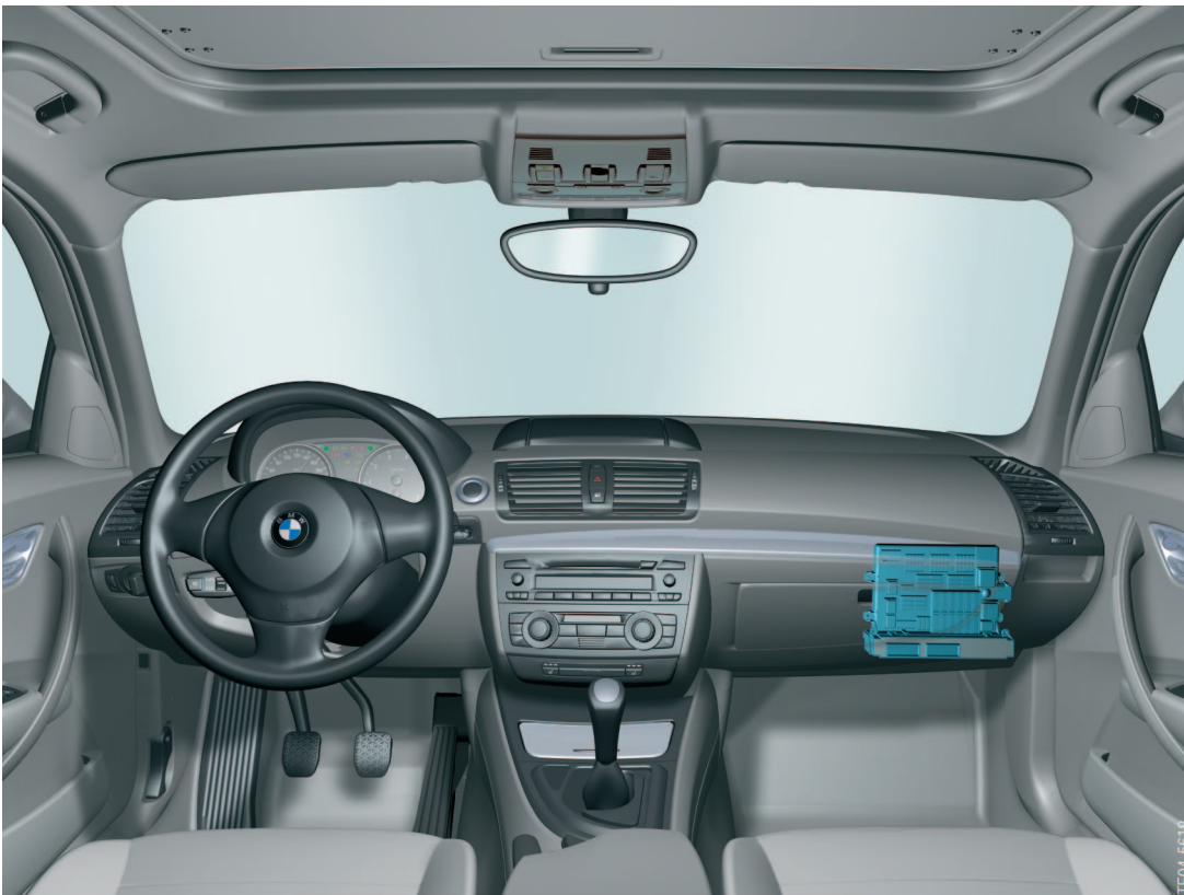
10 - Location of junction box
