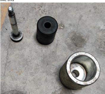
3) After you place the bolt through the shift linkage rod, put the washer that you have ready before inserting the big black bush. Once you put the washer and bush, assembly should look like this –
