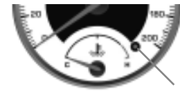
High Temperature Warning
