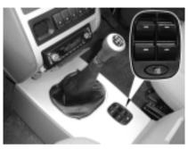
Switches on the central console for operating the door glasses
