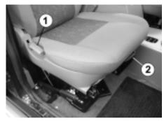
Seat backrest inclination adjustment lever
