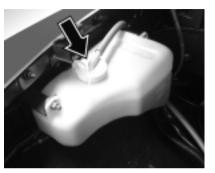
Engine Coolant Auxiliary Tank
