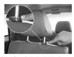
Release Button for Head rest height adjustment
