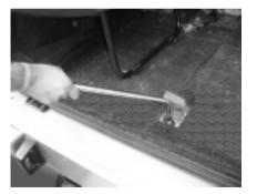
Loosening/Tightening of wheel winch screw
