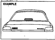
High mount stop lamp is provided with your vehicle and is fitted on rear parcel tray. The stop lamp will glow as when the brake pedal will be depressed.
