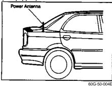
Power antenna on the rear side will automatically come up on switching on the AM/FM receiver fitted in the vehicle.
