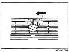
Push the under-bonnet release lever sideways with your finger, as shown in the illustration. While pushing the lever, lift up the bonnet.
