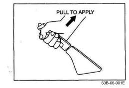
The parking brake lever is located between the seats. To apply the parking brake, hold the brake pedal down and pull the parking brake lever all the way up.
