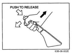
To release the parking brake, hold the brake pedal down, pull up slightly on the parking brake lever, push the button on the end of the lever with your thumb, and lower the lever to its original position.
