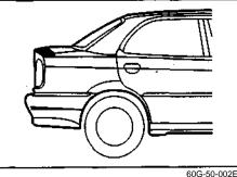
Rear Spoiler is provided to improve aerodynamic stability at higher speeds and better asthetics. Stop Lamp (if equipped) is fitted inside the Rear Spoiler. The stop lamp will glow as and when the Brake Pedal is depressed.
