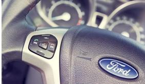
Steering mounted controls with SYNC
