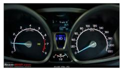
Silver Instrument panels Instantaneous mileage indicator Avg. Mileage indicator Tachometer Distance to empty Avg. Speed
