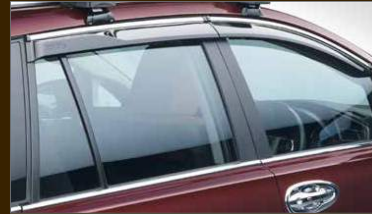
Side Visor with Chrome allows you to leave the window slightly open when its raining
