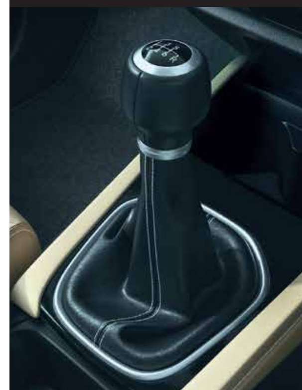
6 SPEED MT FOR 1.5 Litres i-VTEC & i-DTEC ENGINES
