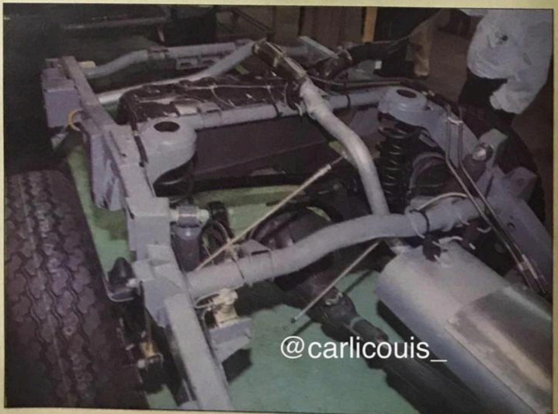
The ladder type chassis frame (with eight cross members) owes its ancestry to the 207 family. While torsion bar sprung independent front suspension is employed, the rear layout (pic) employs the five link layout as seen on the Sierra.
