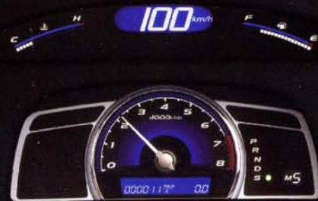
Multiplex Meter reduces eye movement
