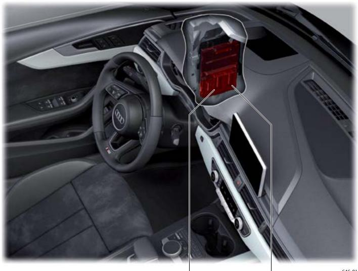
Connector C (54-pin) to cockpit wiring harness 646\_012
