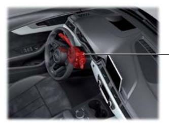
Steering Column Electronics Control Module J527
