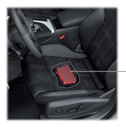
Memory Seat/Steering Column Adjustment Control Module J136
