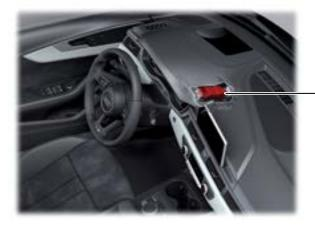
Electronic Steering Column Lock Control Module J764
