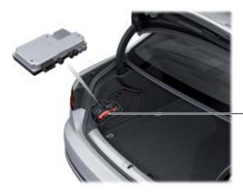
Peripheral Camera Control Module J928
