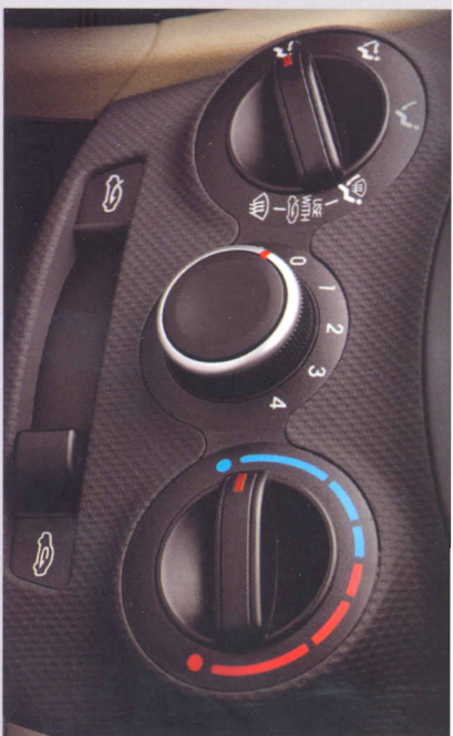
Manual Air Conditioner This convenient and instantly recognizable triple dial knob lets you control and adjust the temperature and airflow according to your need.
